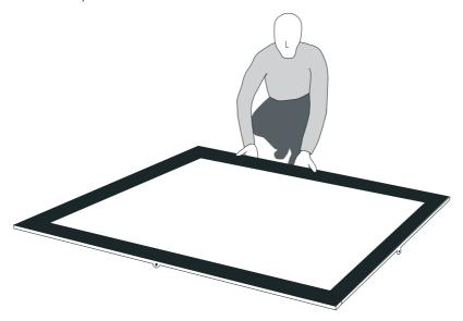
The screen support frame is supplied with magnetic tape on the rear. The screen is applied up to the magnetic bars on the Premier P300 U-shaped frame.
