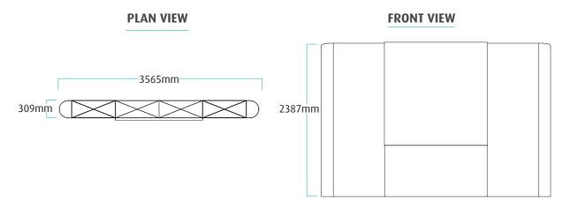
The smaller sized CK is based on a 3 X 4 Premier P300 flat frame. This accommodates a 2 X 2 quad projection screen.
